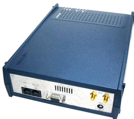
Figure 1.1 La passerelle RNIS-GSM
